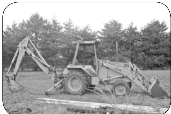
Case Super 580E Backhoe
