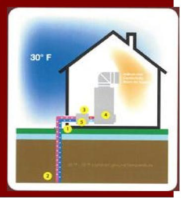
ETA Geothermal unit sends an environmentally friendly cold refrigerant (R-410A) into a patent copper <sup>(B)</sup> based ground source heat exchanger (CGSHE)."
